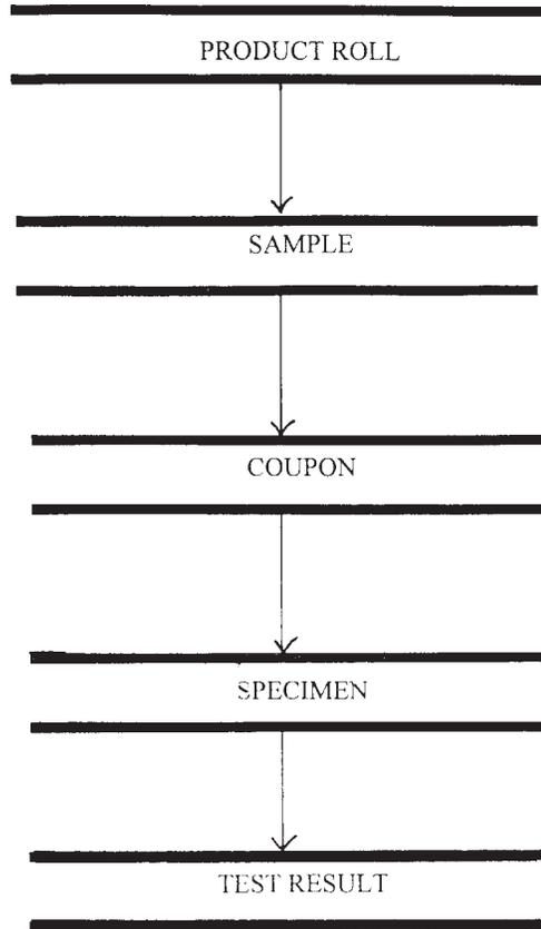
NOTE 1—Product roll is from the manufacturer. Samples are cut from the product roll. Coupons for outdoor exposure are cut from samples. Specimens for tensile testing are cut from coupons.
